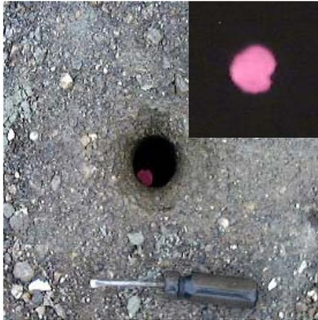
Photo shows combusting wastes at the location of a former landfill gas extraction well. Insert is close up.
